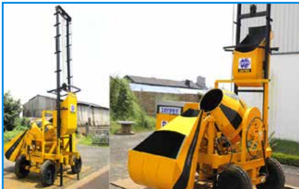
Concrete mixer & hoists
